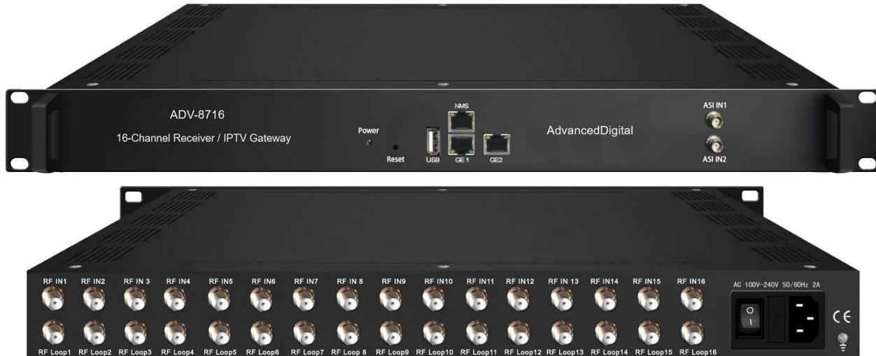
The ADV-8716 is a high-density Receiver / IPTV Gateway equipped with 16 independent RF tuners, these can either one of DVB-S/S2, DVB-C/T/T2, ISDB-T and ATSC. It is also equipped with 2 ASI input ports.
