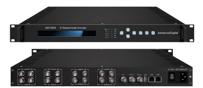
ADV-8608 is a professional audio encoder with powerful functionality. It has 8 independent channels of unbalanced audio inputs supporting MPEG 1 Layer II compression. Furthermore, it supports audio gain control in a wide range. ADV-8608 outputs encoded audio through both ASI and IP ports for further transmission.
