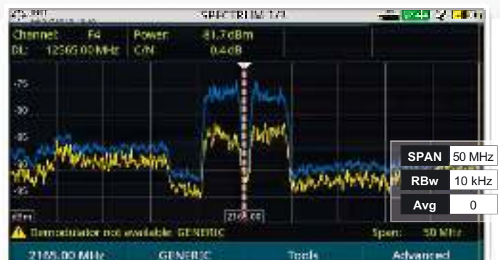
2.1 GHz Terrestrial Interference from mobile phone base station
